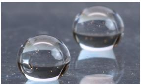
Developed specifically for aviation applications, ice protection NPL uses proprietary nanotechnology to create a super-hydrophobic surface on existing substrates that can repel water and drastically minimize ice buildup. In addition, ice protection NPL provides excellent corrosion protection for the substrate.
